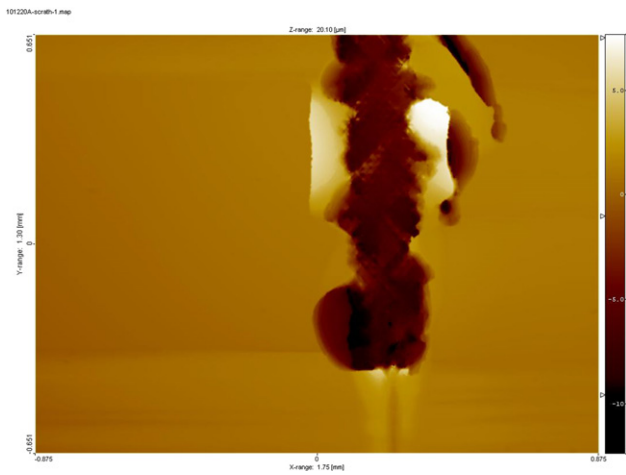
Figure 8. Micrograph of the scratch track with critical load.
